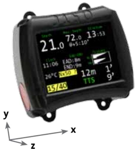
OSTC 2 has a tilt-compensated electronic compass. Like all other electronic compasses it must be calibrated before use. The calibration compensates aberration that can be caused by the battery. It is recommended to compensate the compass if your dive computer shows big deviations in the heading reading.
