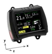
OSTC 2 has a tilt-compensated electronic compass. Like all other electronic compasses it must be calibrated before use. The calibration compensates aberration that can be caused by the battery. It is recommended to compensate the compass if your dive computer shows big deviations in the heading reading.
