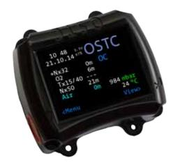
heinrichs weikamp delivers the OSTC 2 ready for use with a high quality rechargeable lithium battery. Anyway we recommand to load the OSTC 2 completely before you use it the first time.
