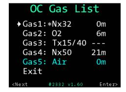
Use **OC** gas setup to configure presets for up to five gases for scubadiving as well as bailout gases for rebreather diving . You can switch between these presets when you change your gases while diving.
