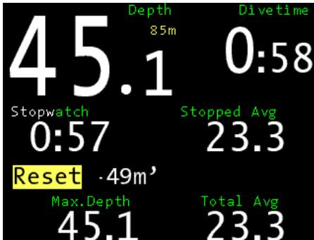
With »Reset« (left button) the stopwatch is restarted and the stopped average depth (Stopped Avr) is displayed.
